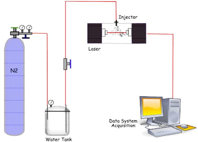
**Figure 1** Experimental apparatus of the atomizer system.
