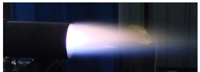
Figure 1 Burning Condition of Minimal- oil Gun on Laboratory Bench
