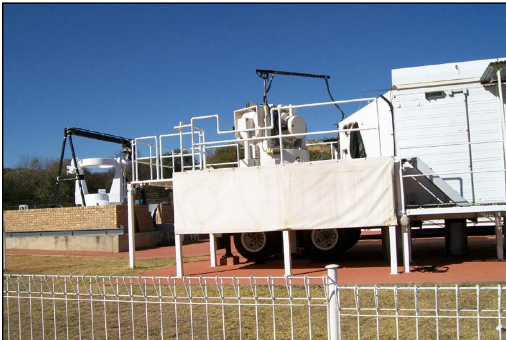
Figure 61. The Lunar Laser Ranger (LLR) is currently being developed at HartRAO (left) and MOBLAS-6 SLR station (right). Once the development is completed, the LLR station will be moved to Matjiesfontein.
