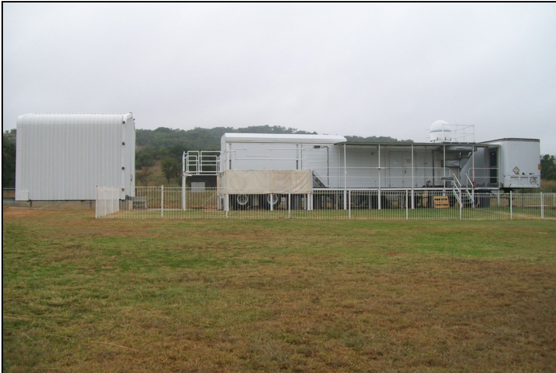
Figure 8. Collocated geodetic instruments at HartRAO, South Africa. Left: LLR/SLR station under development; Right: SLR (MOBLAS-6) station, due to bad weather the telescopes are closed up.
