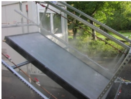
Fig. 5: The rain penetration test.
