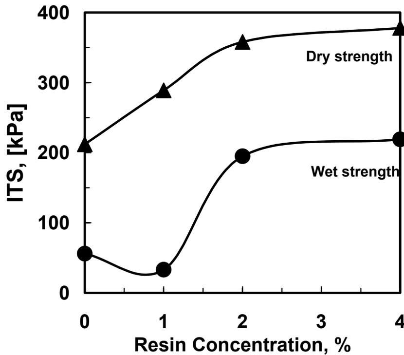
Figure 6: Effect of resin concentration on the dry- and wet strengths of a soil containing 2% anionic bitumen emulsion. Resin pH was adjusted to pH = 4,5 and soil moisture content to 10%. Samples were dried in air for 21 days before being subjected to dry and wet strength testing.
