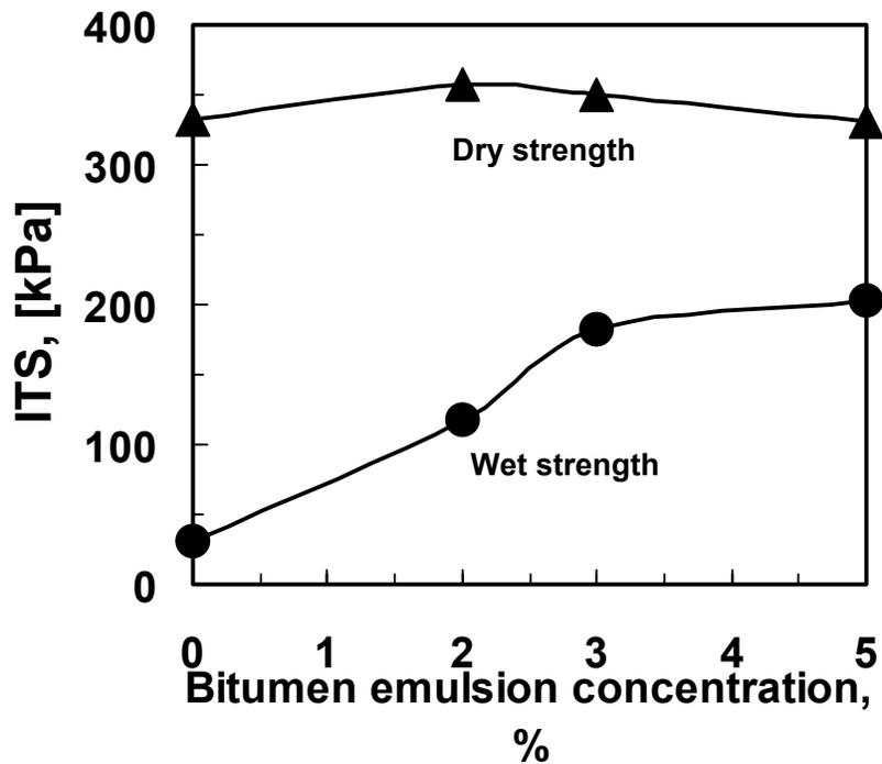
Figure 7: Effect of anionic bitumen emulsion concentration on the dry- and wet strengths of the soil containing 2% resin. Resin pH was adjusted to pH = 4,5 and soil moisture content to 10%. Samples were dried in air for 21 days before testing.
