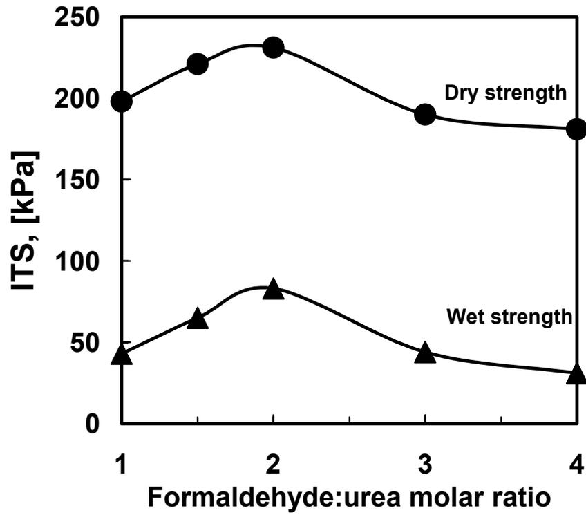
Figure 5: The effect the reactant stoichiometry on the 7-day strengths of soil stabilised with 2% UF resin and 2% anionic bitumen emulsion. The soil moisture content was set at 10% and the resin pH adjusted to pH = 4,5.
