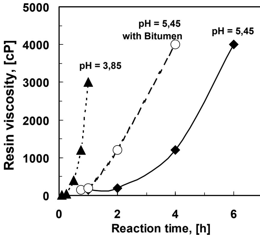
Figure 3: The influence of pH and anionic bitumen addition on the viscosity of the resin during curing at a temperature of 25°C. The formaldehyde:urea molar ratio was 1,23:1. The bitumen emulsion was SS60 added at a 1:1 mass ratio.
