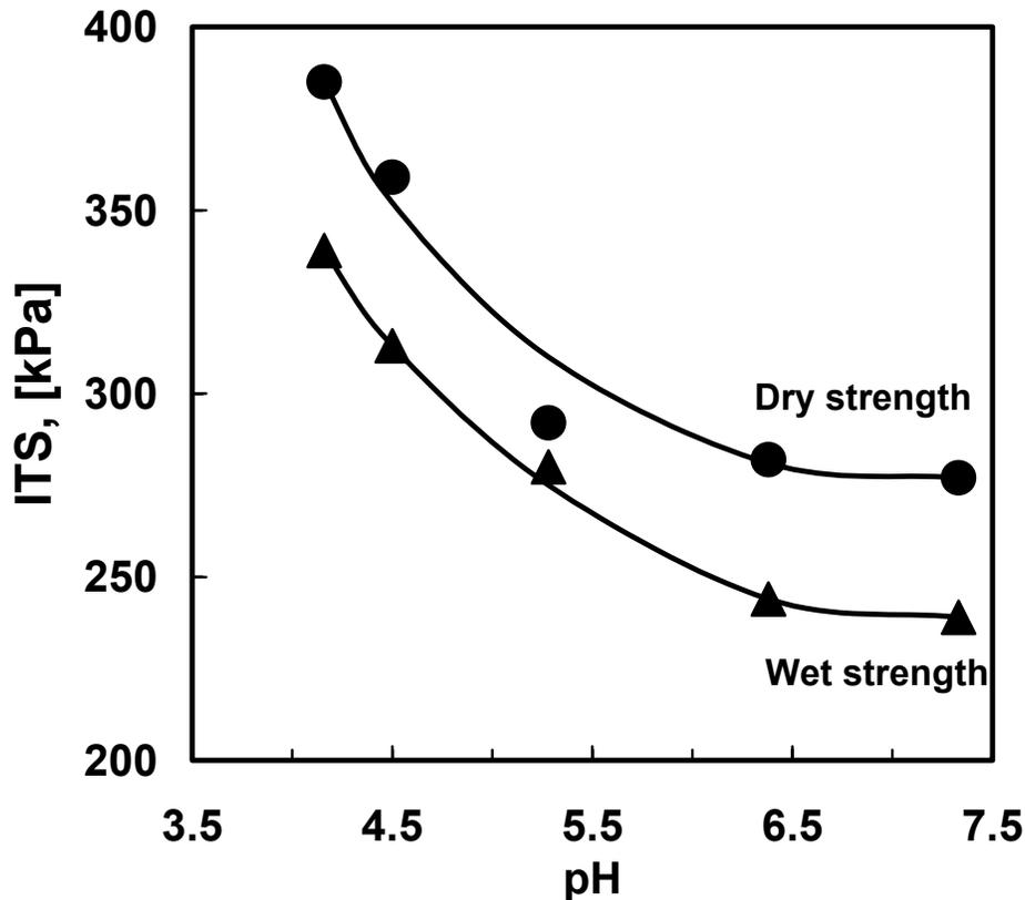
Figure 4: The effect initial resin pH on the 7-day strength of soil stabilised with 2% UF resin and 2% anionic bitumen emulsion. The initial soil moisture content was set at 10%.
