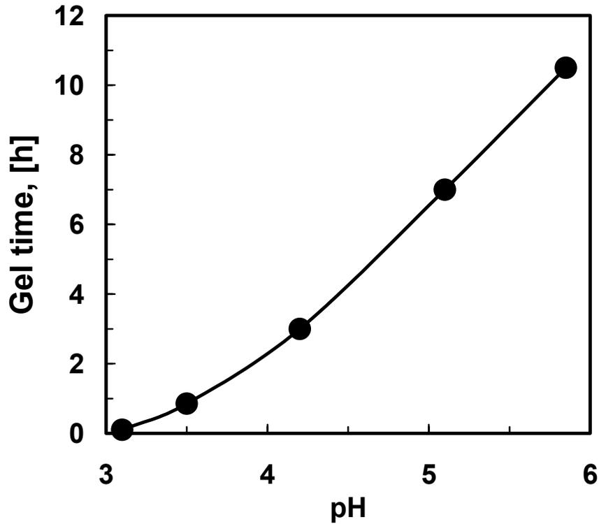
Figure 1: The effect initial resin pH on geltime at 25°C for a resin with a formaldehyde:urea molar ratio of 1,25:1.
