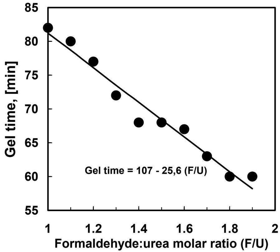
Figure 2: The influence of the formaldehyde:urea molar ratio on the resin gel time at a temperature of 25°C and pH =3,9.
