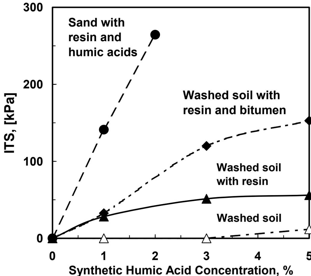
Figure 9: Effect of synthetic fulvic acid addition on 7-day dry strength of soils devoid of natural organic substances. Where indicated, UF resin and/or anionic bitumen was added at the 2% level.
