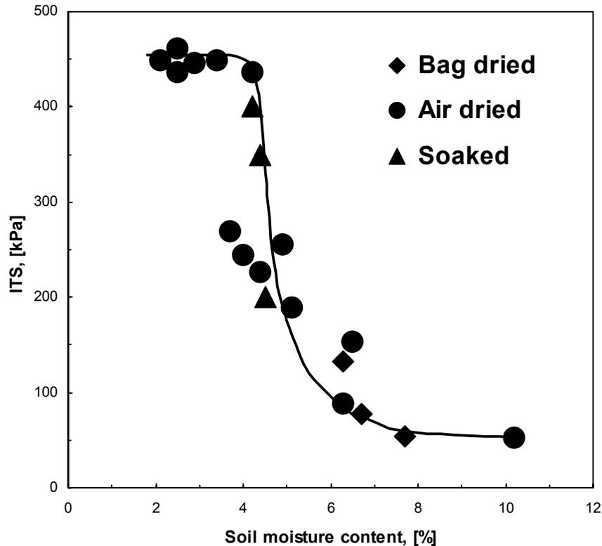
Figure 8: The effect of the final moisture content on the strength of soil stabilised with 2% UF resin and 2% anionic bitumen emulsion. The formaldehyde:urea molar ratio was 1,5:1 and the resin pH = 4,5. Samples were either dried in air or cured covered in polyethylene bags.
