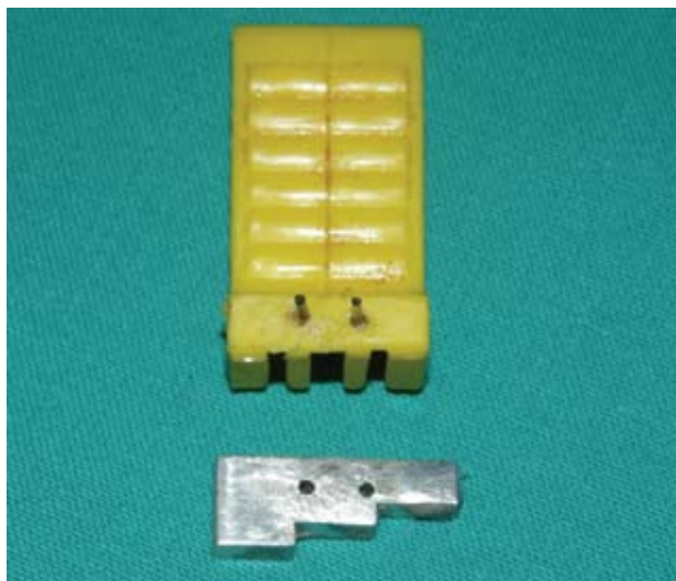
Figure 2: The XPC-DS Digital Position System (e in Figure 1) to which the XPC-DS Digital Systemsensor was fixed and the aluminum step wedge (f in Figure 1) that was used to provide a comparative standard of density, expressed as a gray scale value.
