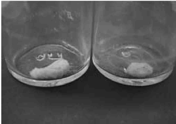
Figure 7 Comparison of different EPS yields following extraction after homogenization with a sonic probe. Samples are from left to right Baviaanspoort and Centurion.
