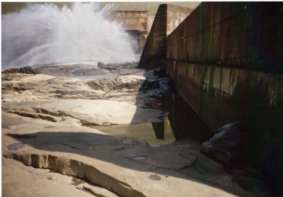
Plate 30 Granitic rock mass with undulating, rough joint planes.
