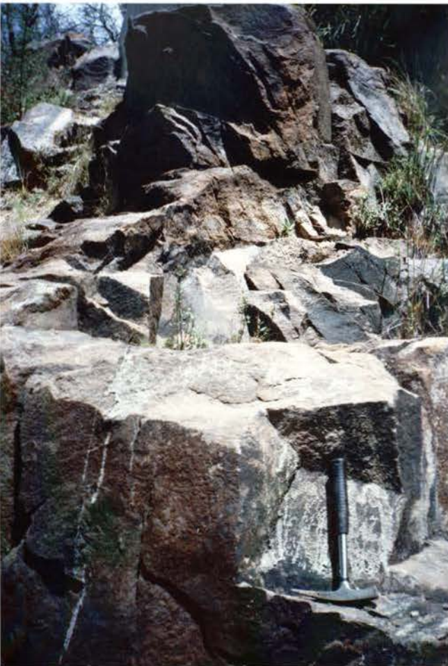
Plate 7 Removable rock blocks formed by slightly continuous, undulating joints.
