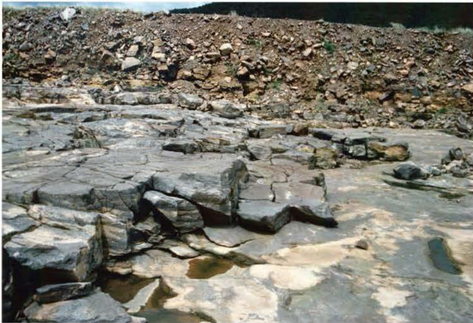
Plate 10 Closely spaced, open joints forming removable rock blocks (Van Schalkwyk).
