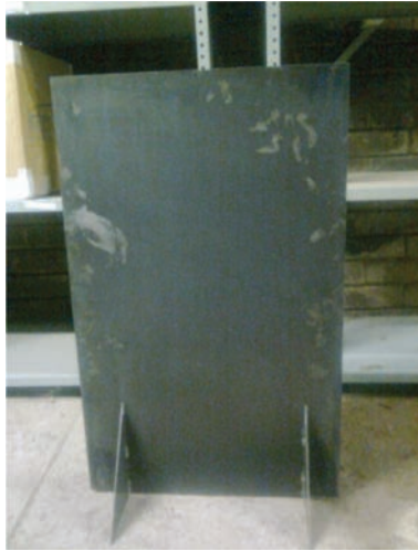
Figure 13—Experimental set-up for measuring the coefficient of restitution
