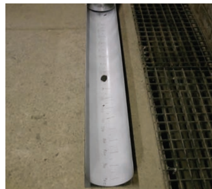
Figure 10—Experimental set-up for measuring the coefficient of rolling friction
