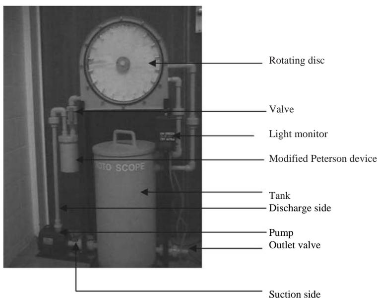
**Figure 1** Laboratory Rotoscope used to monitor biofilm growth
