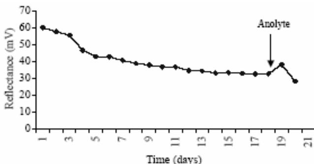
Figure 2 The average reflectance readings as affected by the biofilm on the rotating disc (the arrow indicates the time analyte was added)
