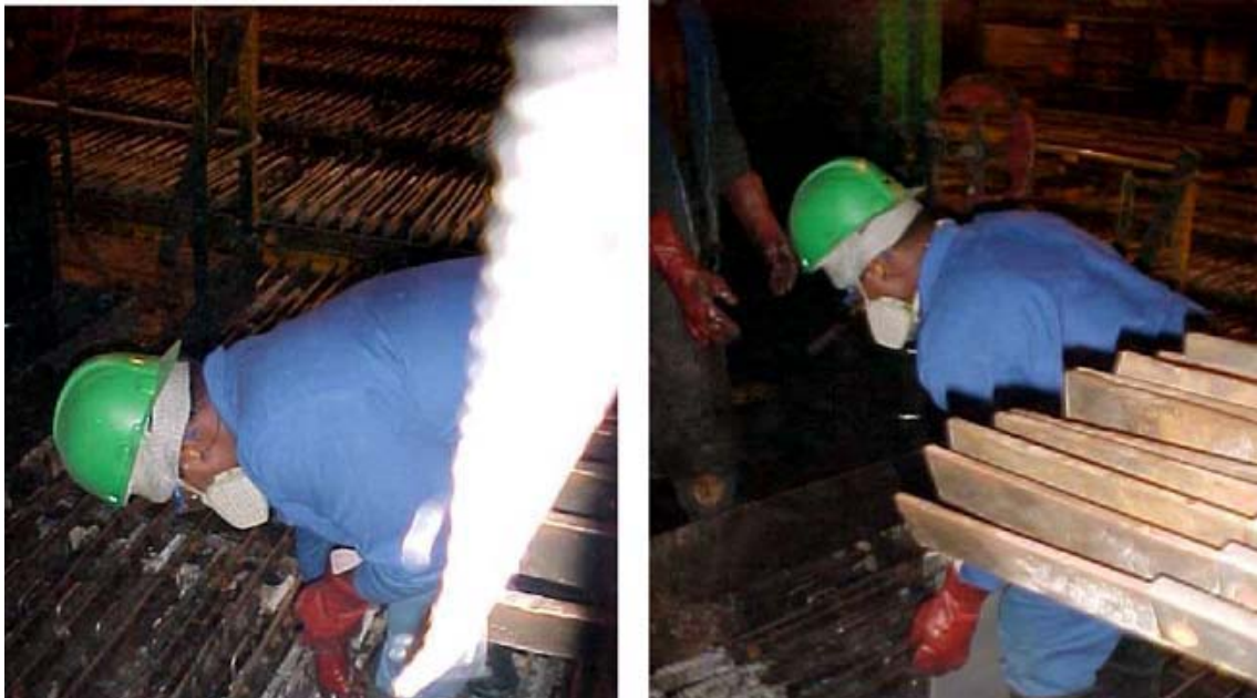
Fig. 2 Cell house worker stripping plates
