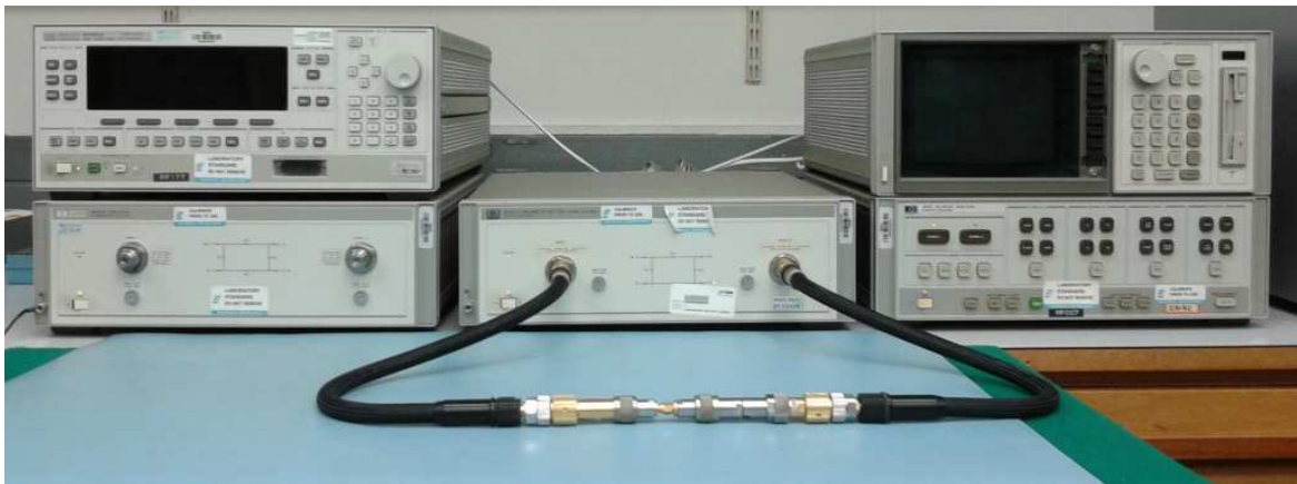
Figure 3.10. Photograph of the adapters connected to the VNA.
