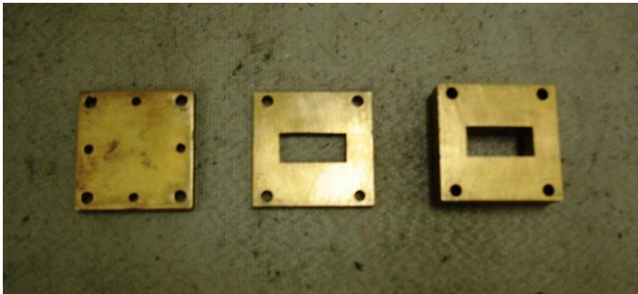
Figure 5.2. Two X-band delay plates together with the Short plate used for the experiment.
