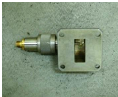
Figure 5.1. Siverts Lab PM 7325X X-band mode transformer with an N-type to SMA adapter.
