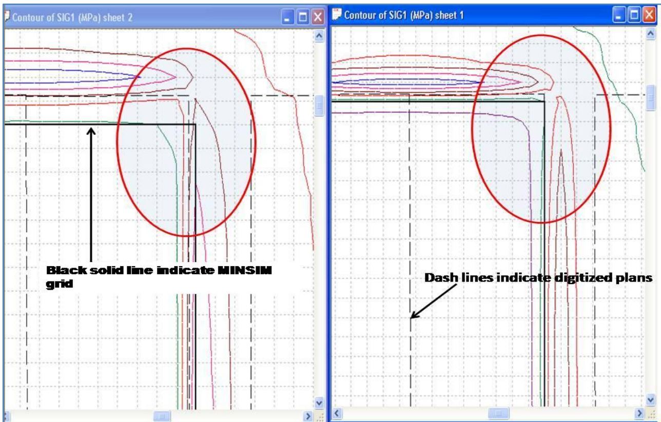
Figure 62: Difference of calculating major principal stress when the grid position was not set (line contour plots)
