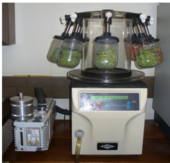
Figure 3.1: Freeze-dryer used to dry C. orbiculata , B. volubilis and M. plumbea plant material.
