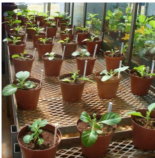
Figure 6.2: A randomized block design of the N. tabacum plants for the phytotoxicity test.
