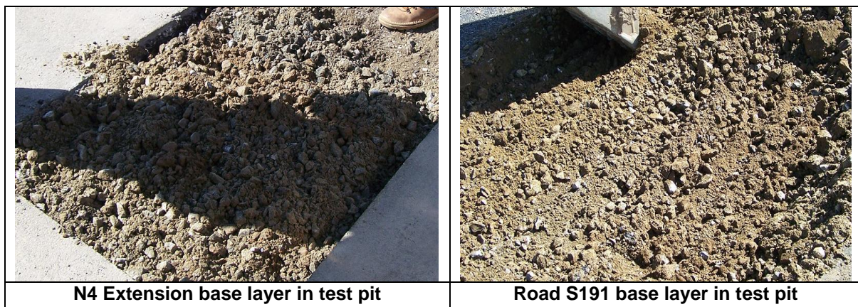
Figure 5.1: Bulk samples of base layer material from N4 Extension and Road S191.
