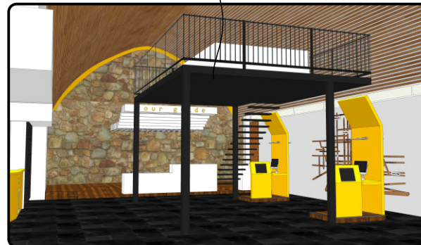
steel portal structure cladding in corian
