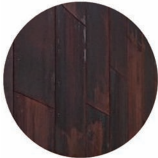
WEATHERING STEEL CLADDING
