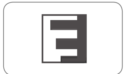
Jointed - 360° view; security integrated in surrounding buildings; makes it easier for the guard to reach all areas.
