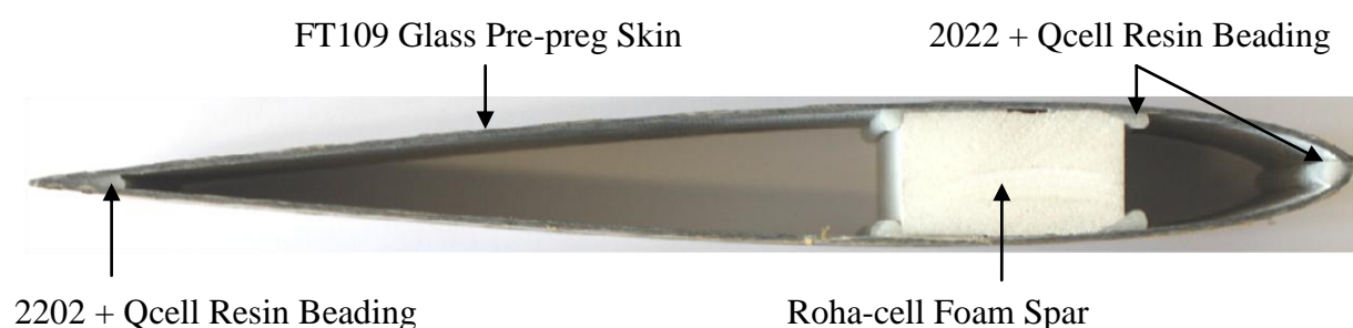
Figure 3-4: Composite Wing Construction
