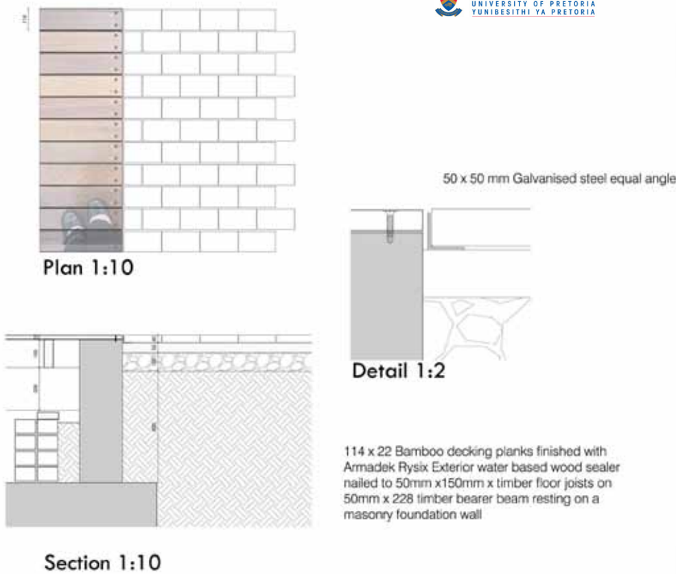
Figure 8-33 DETAIL: paving -deck threshold (Author, 2013)
