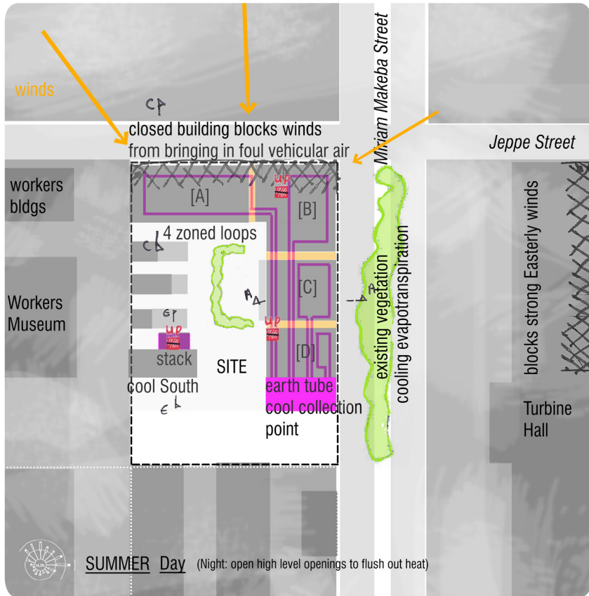
Figure 118: Schematic plans of passive ventilation systems [Author, 2013]
