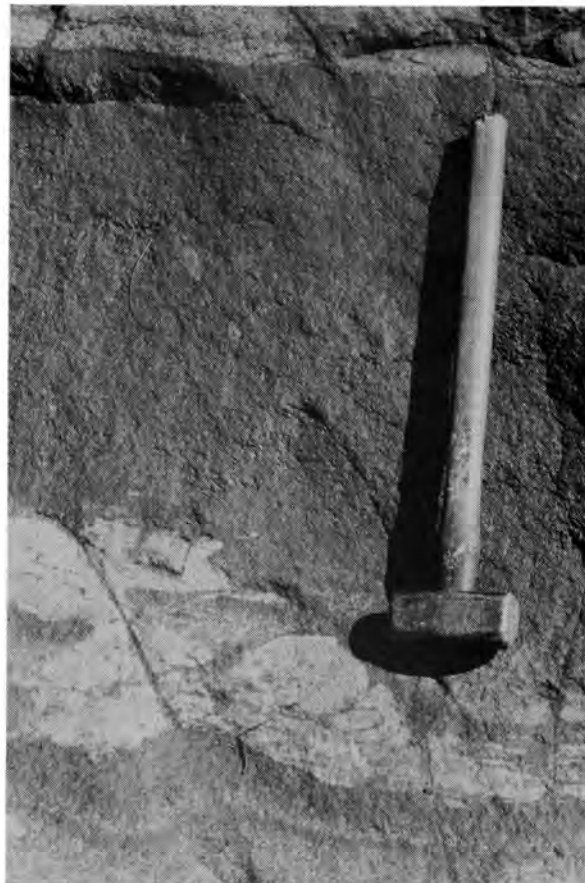
Fig 22. Magnetite Seam 19, characterized by a sharp upper contact, gradational lower contact and irregularly shaped inclusions of anorthositic material at its base. Onverwacht 148 JS.
