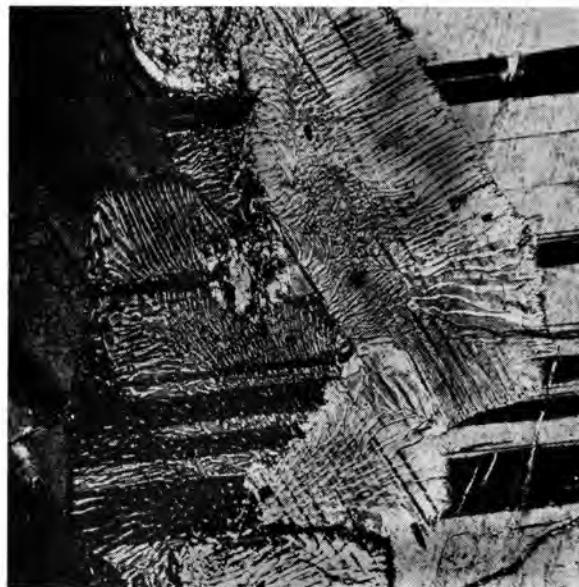
Fig. 49. Crystal of plagioclase completely transformed to myrmekite (centre). G609. Crossed nicols, x75
