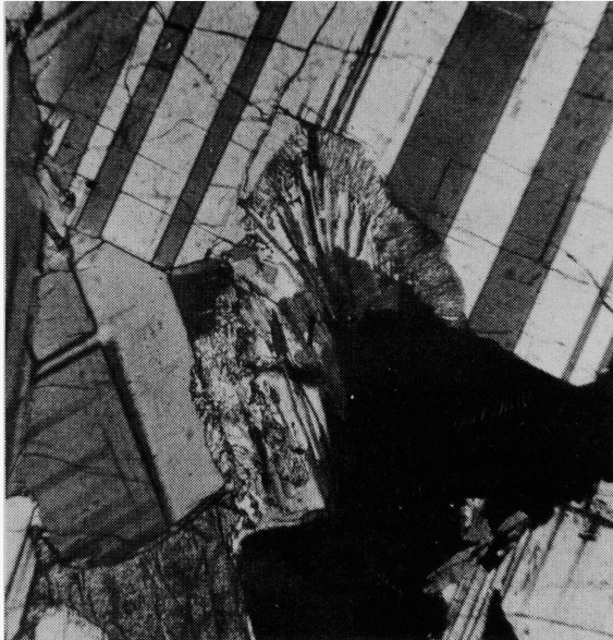
Fig. 61. Complex symplektite which consists of an inner zone (dark grey) of biotite, a central zone of "needles" of biotite in plagioclase and an outer zone of myrmekite-like intergrowth of pyroxene and plagioclase. G396. Crossed nicols, x70.
