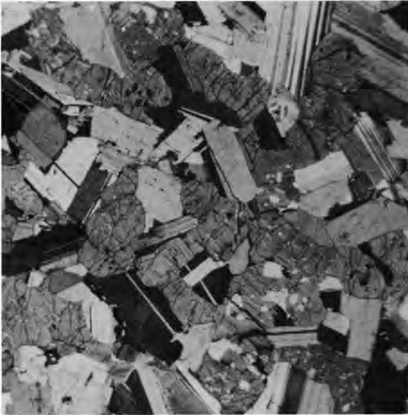
Fig. 36. Similarly orientated crystals of orthopyroxene (grey) which contain a few blebs of exsolved augite. G589, Uysedoorns 47 JT. Crossed nicols, x20.
