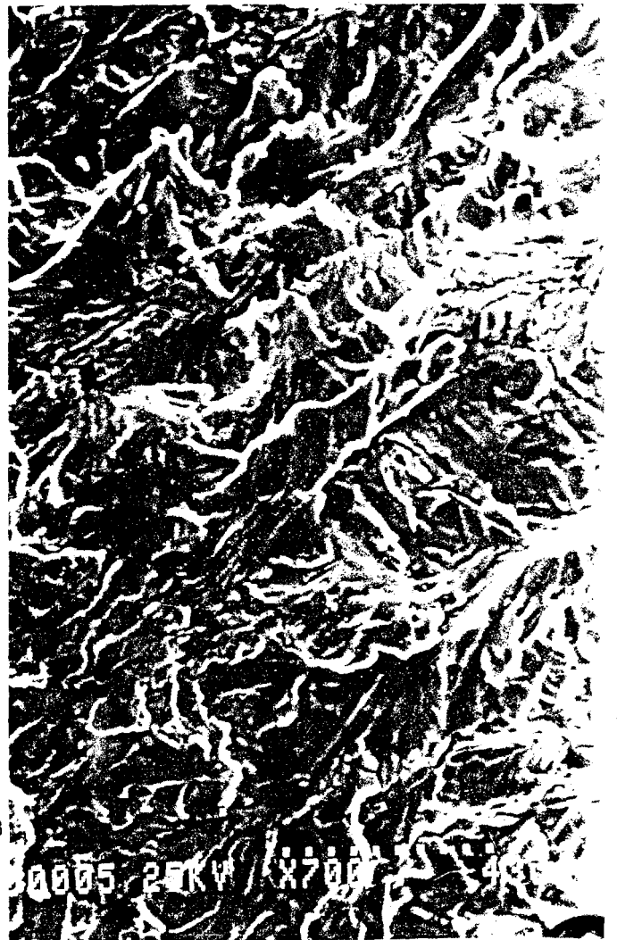
FIGURE 71 Fracture surface of CERT specimens tested in rich gas.
