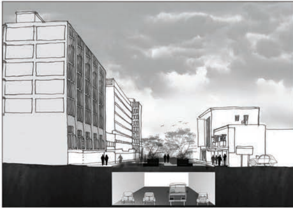
Figure 80. Submerged road with pedestrian link on street level (Author, 2012).
