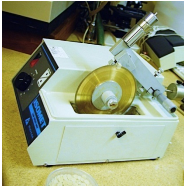
Fig. 3.3: A representative photograph of a central maxillary incisor being decoronated by a diamond wafering blade in an Isomet 11 – 1180 low speed saw
