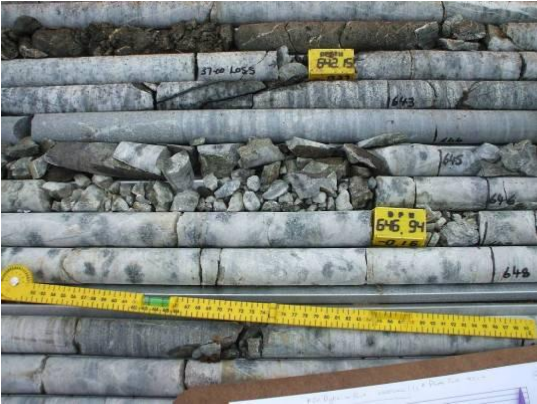
Figure 44: WF49 fault affected area.
