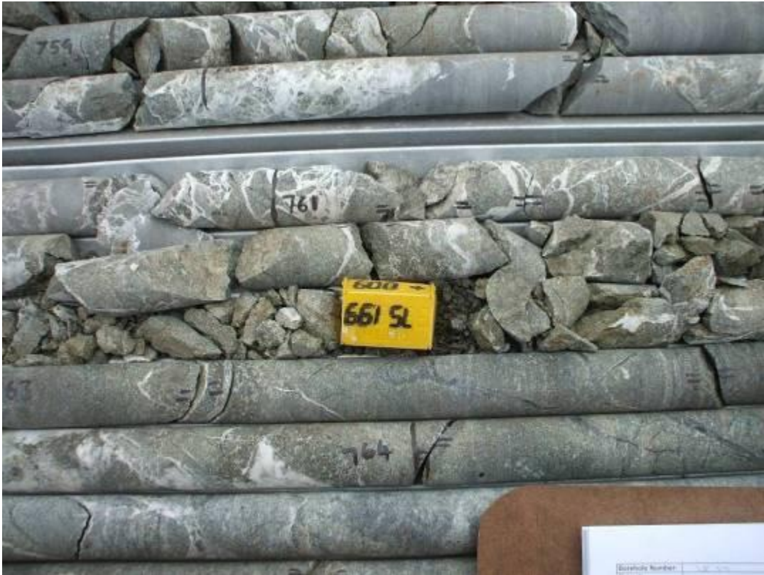
Figure 48: WF59 fault affected area.
