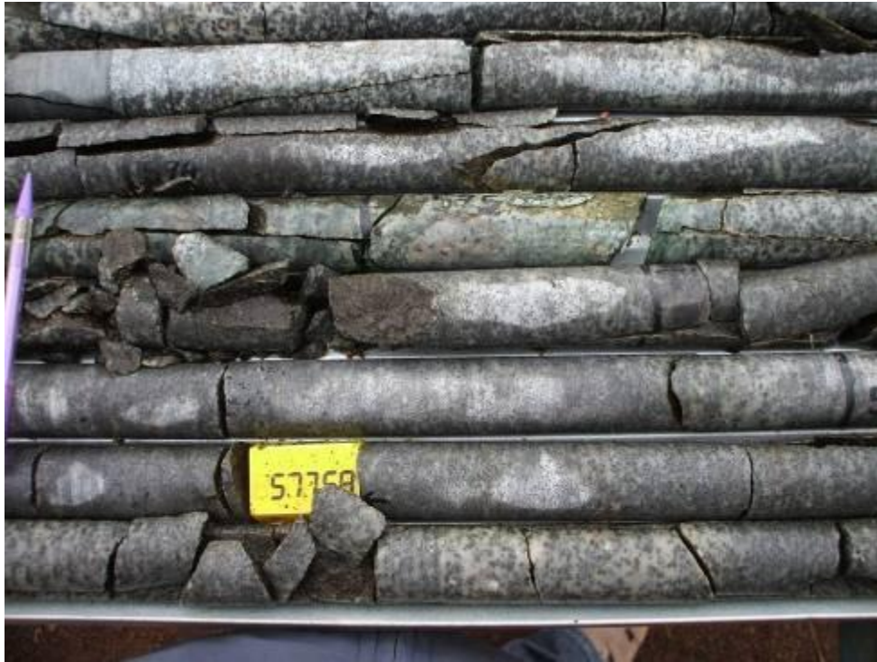
Figure 42: WF1 fault affected area.
