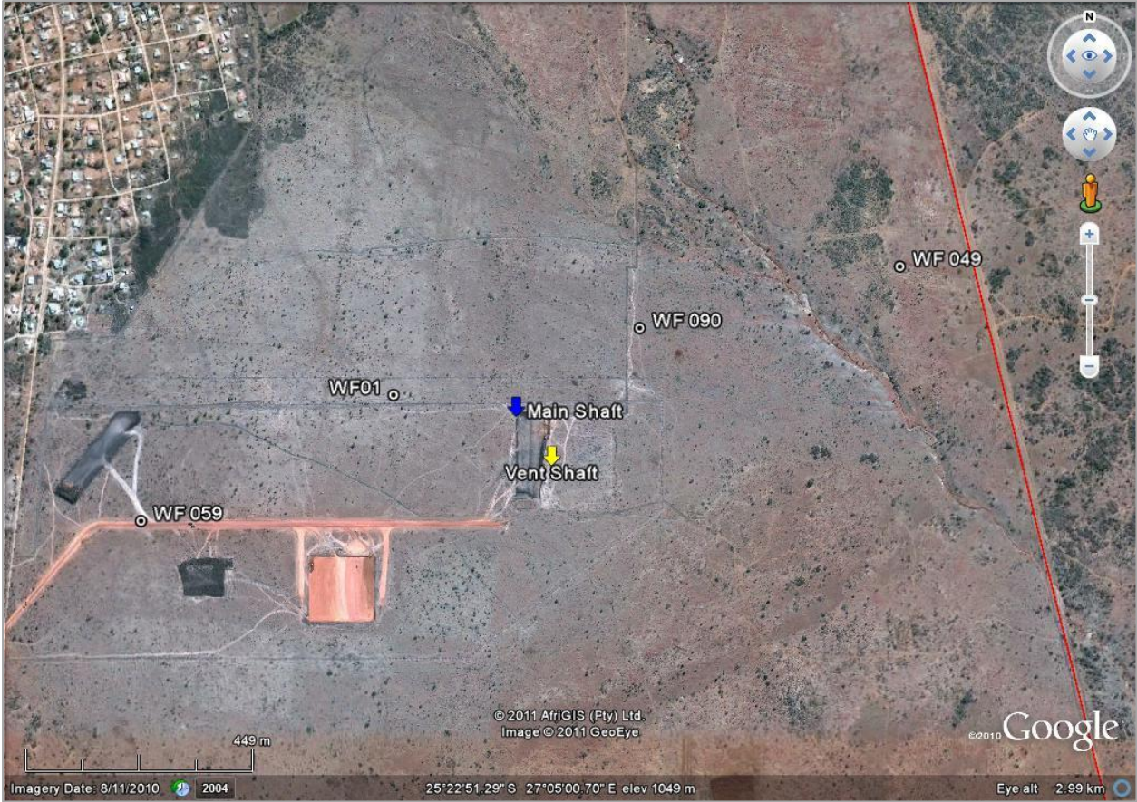
Figure 2: Google Earth image showing the positions of the boreholes that intersected the fault (note the town of Ledig to the west and lease boundary in red to the east).
