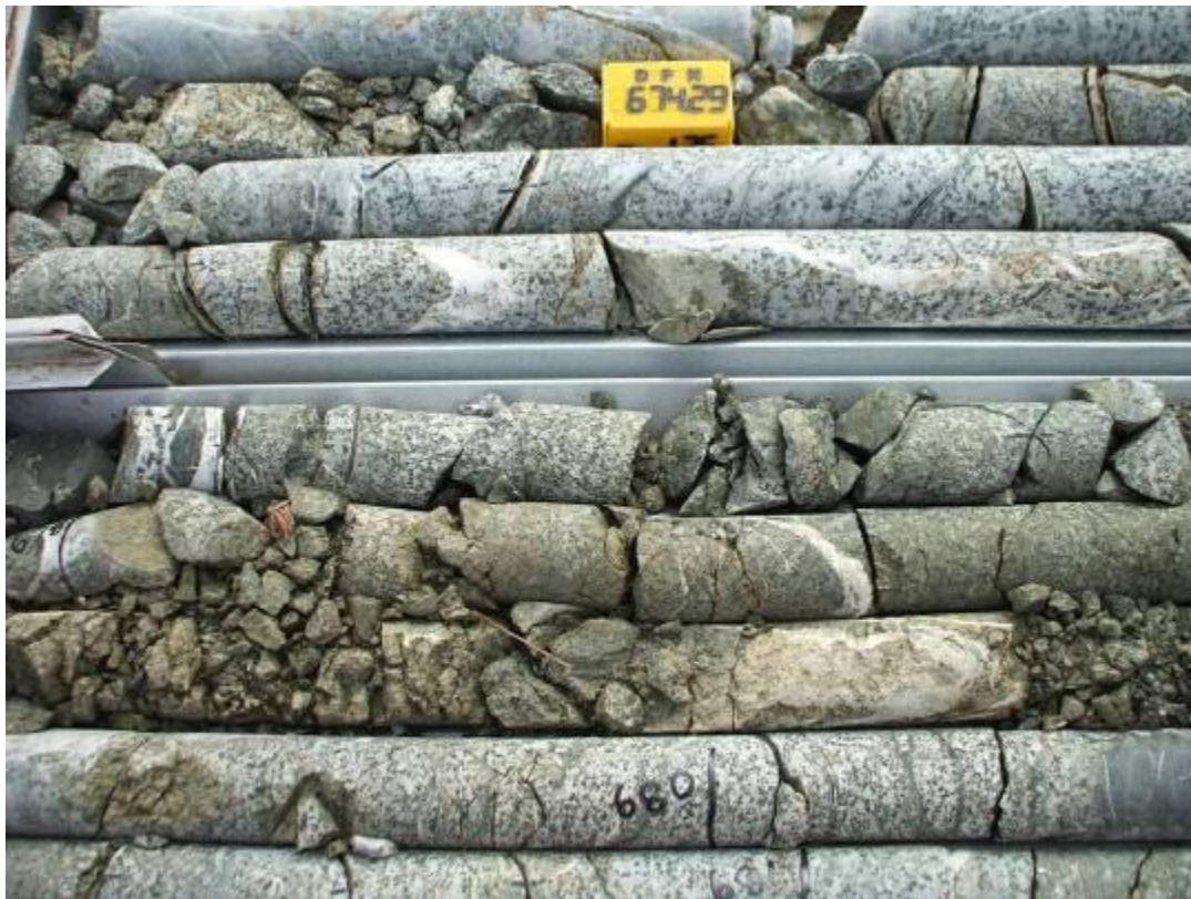
Figure 49: WF90 fault affected area.
