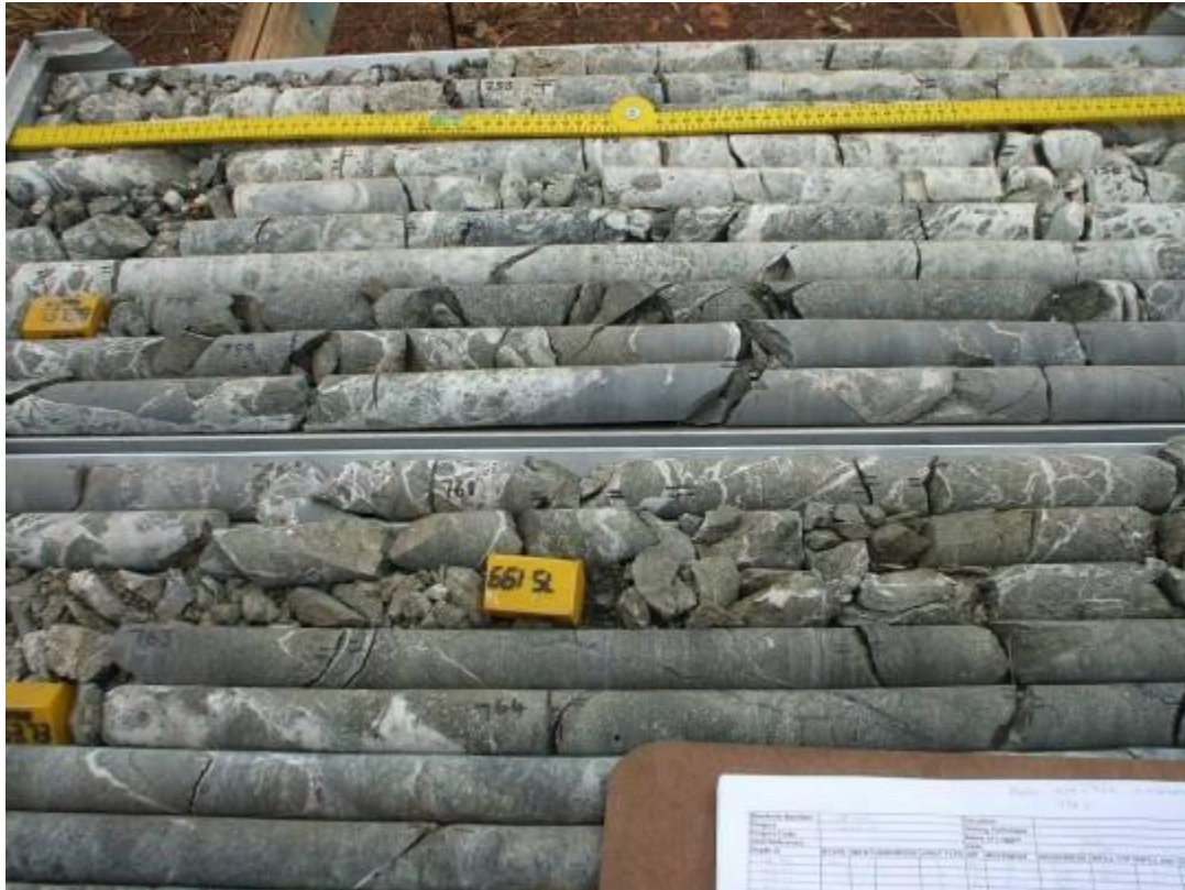
Figure 46: WF59 fault affected area.
