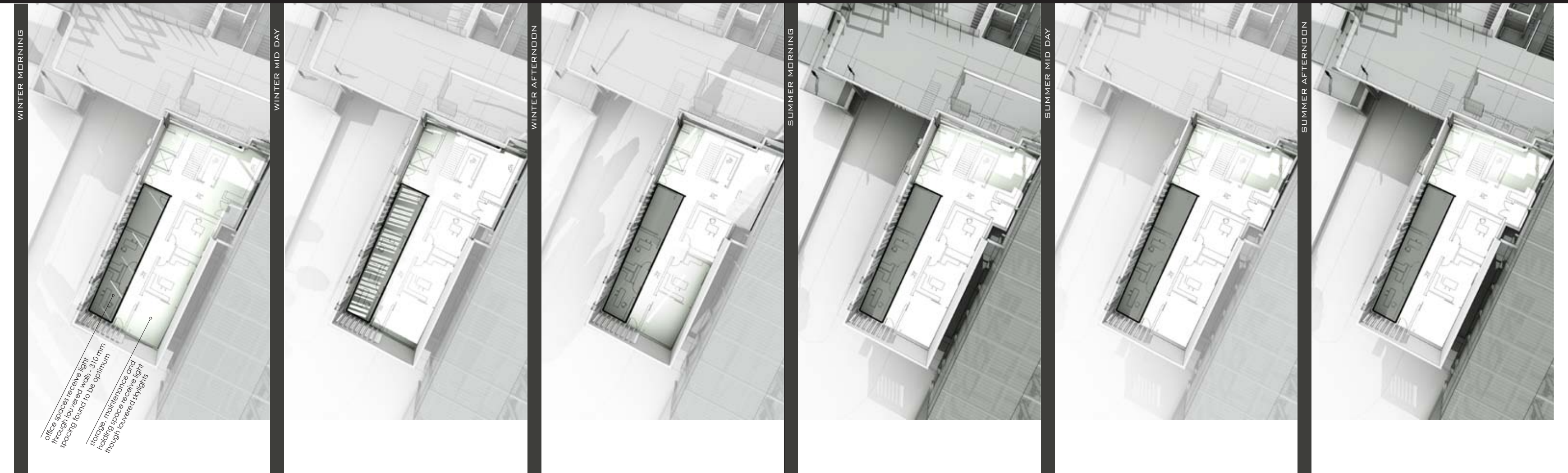
Figure 10-48 Mapping of solar access through louvers at 310 mm spacing, by author (Oct 2012)
