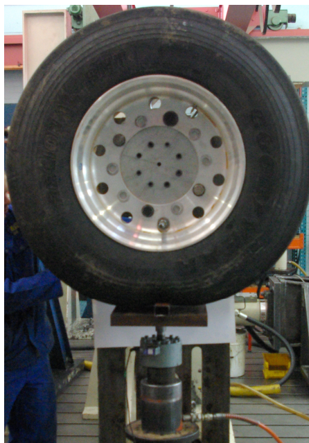
Figure 2.8. Experimental setup to determine tyre stiffness.
