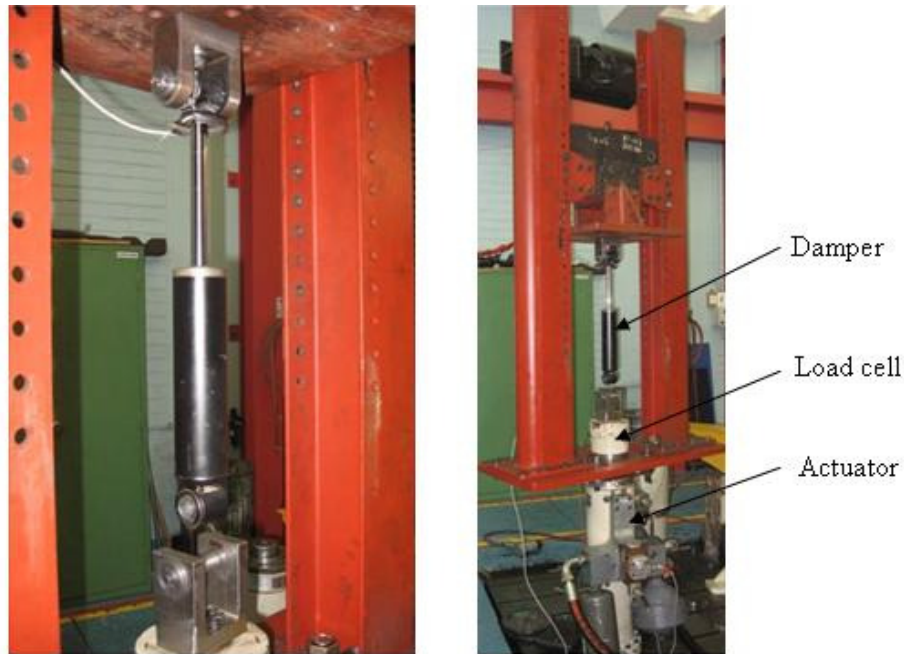
Figure 2.1. Experimental setup for damper characterisation and calibration.
