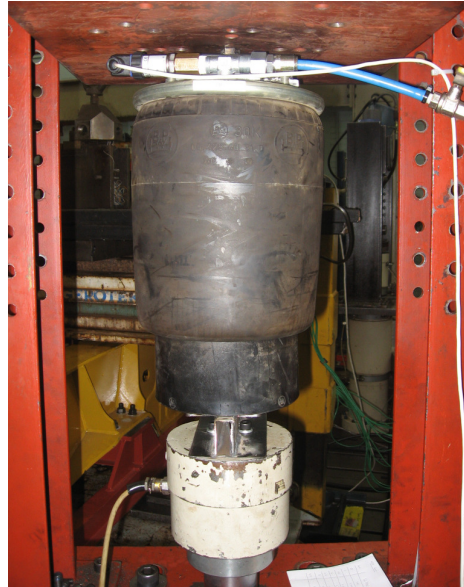
Figure 3.14. Experimental setup for characterising the air spring.
