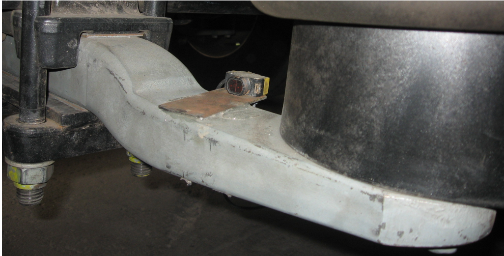
Figure 2.14. Optical sensor for speed measurement.
