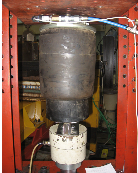
Figure 2.5. Experimental setup for characterising the bump stops.
