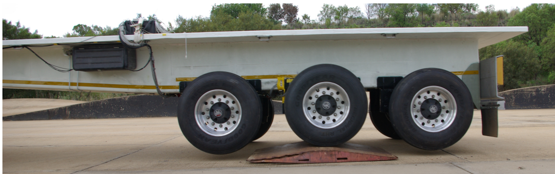
Figure 2.17. Trailer driving over the trapezoidal speed bump.
