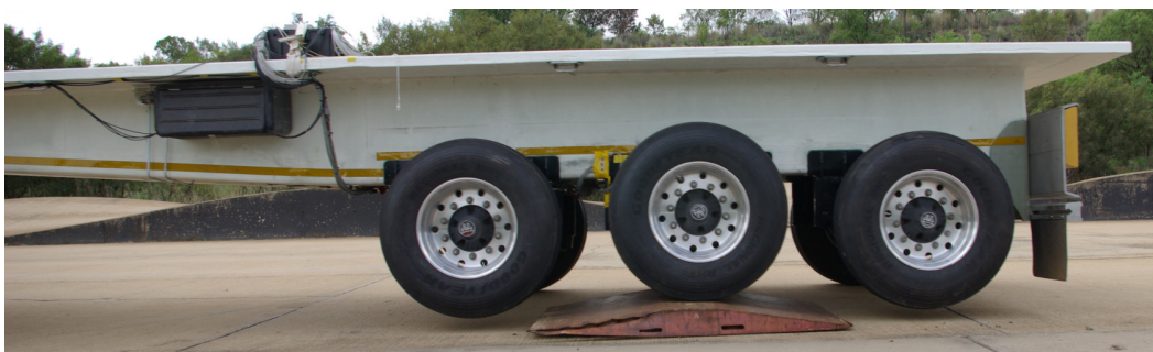
Figure 4.15. The asymmetrical discrete obstacle.
