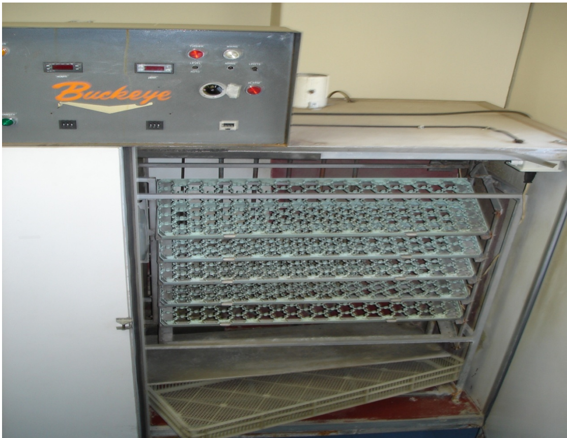
Fig. 3.6. The incubator measures temperature and humidity using electronic detectors. The eggs were incubated and the hatching boxes placed at the bottom (Anonymous, 2011d).
