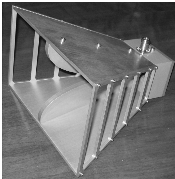
Figure 5.10. New improved 1-18 GHz DRGH antenna.
