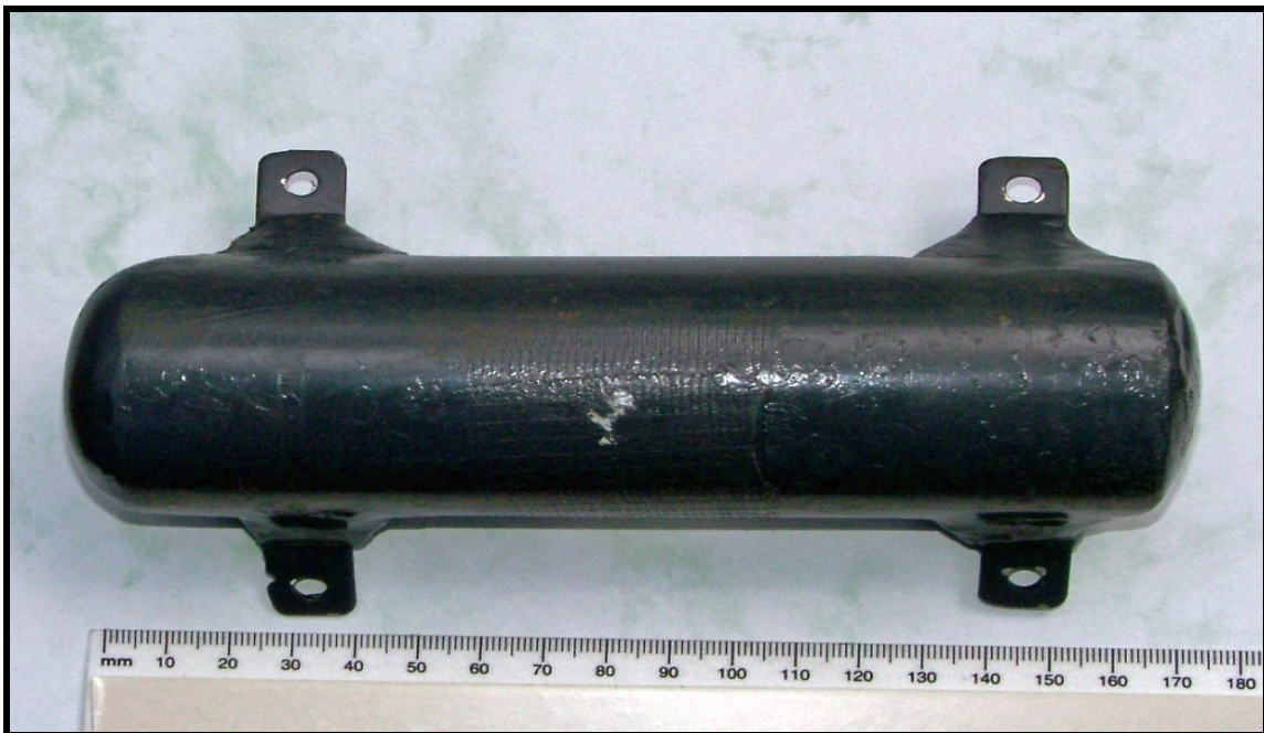
Figure 10: Hawk 105 GPS/GSM transmitter that was used to track the movements of two adult Nile crocodiles in the Flag Boshielo Dam. Note the tabs with holes used for attaching the transmitter to the nuchal scales of a Nile crocodile.
