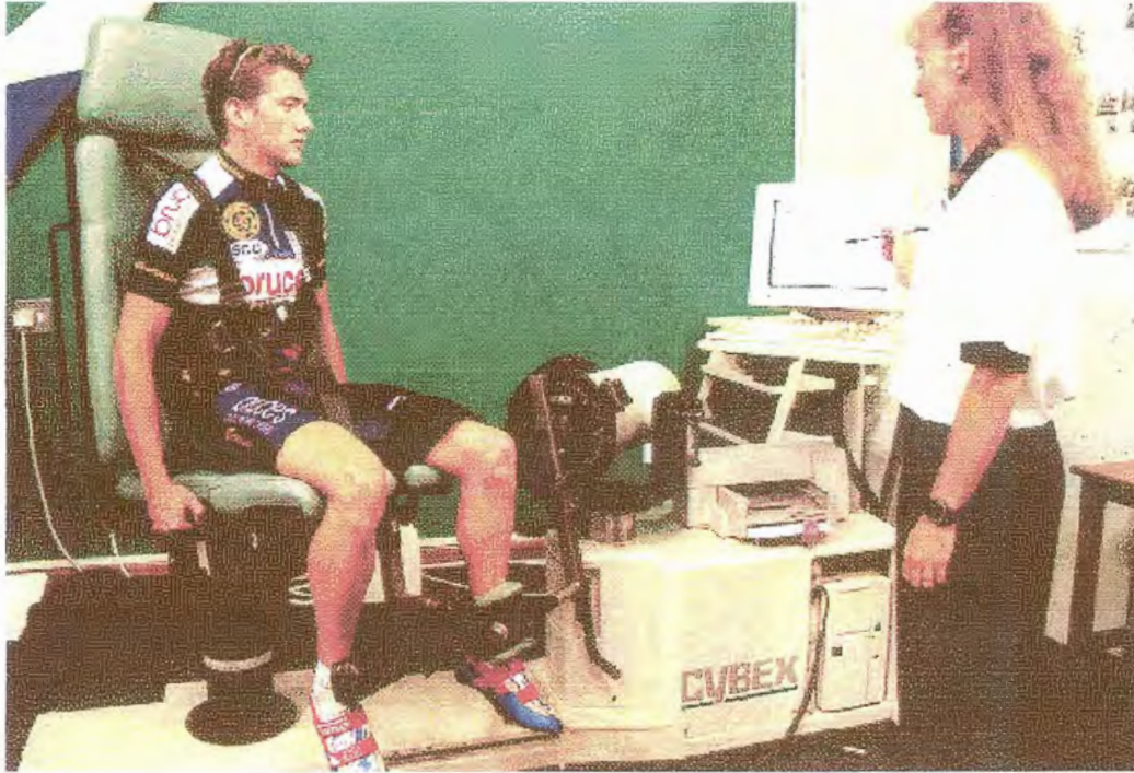
Figure 38: Isokinetic testing on the Cybex Norm
