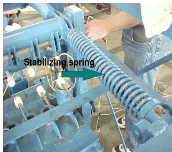
Figure 7.6: Assembly of stabilising springs
