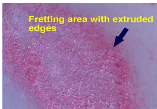
Figure 5.29: Magnification (x 40) of wear on bearing surface area
