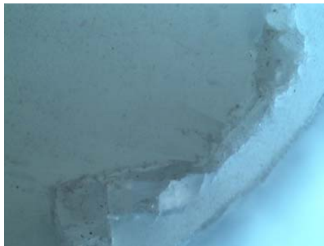
Figure 5.23: Magnification (x 20) of defect on rim of cup
