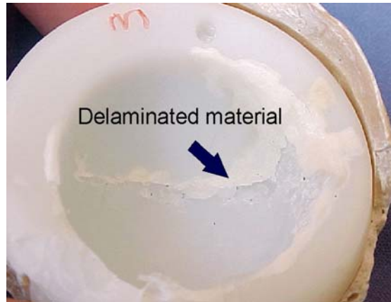
Figure 5.2: A cup with delamination
