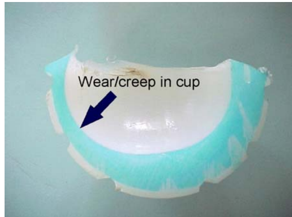
Figure 5.3: Cross section of cups showing an amount of wear/creep
