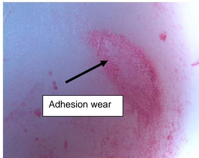
Figure 4.8: Adhesion wear on inside made visible with dye penetrant treatment
