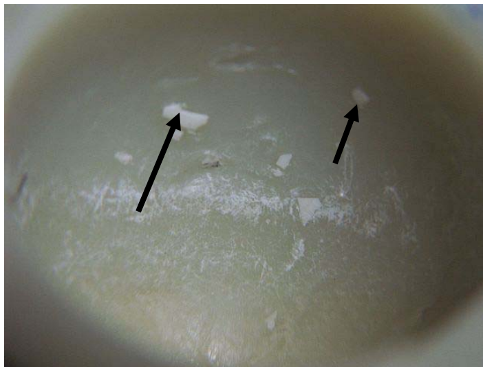
Figure 4.10: Acetabular cup with embedded PMMA particles
