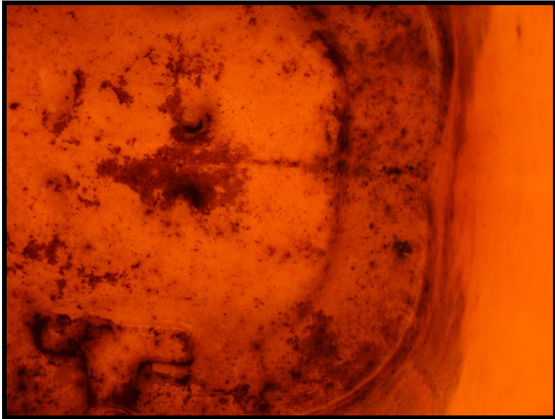
Figure 2.14: Possible contamination route of stored drinking water in rural households in the Vhembe region of the Limpopo Province, South Africa: biofilm formation inside a 25 litre water storage container
