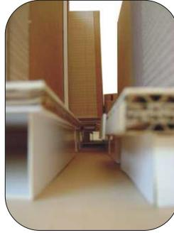
The redesign of the edge with alternating levels visually opens up the arcade. In perspective it seems much wider even though the building edge was not moved back.
