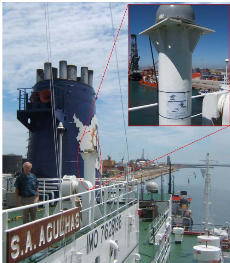
FIGURE 4.1: The position of the GPS antenna relative to the smokestack on the SA Agulhas vessel - with permission from [4].
