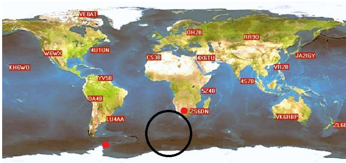
FIGURE 4.37: Locations of the NCDXF/IARU HF beacons. The black circle indicated the operating region of the SA Agulhas research vessel. Taken from the NCDXF HF Beacon Project web site, with permission.
