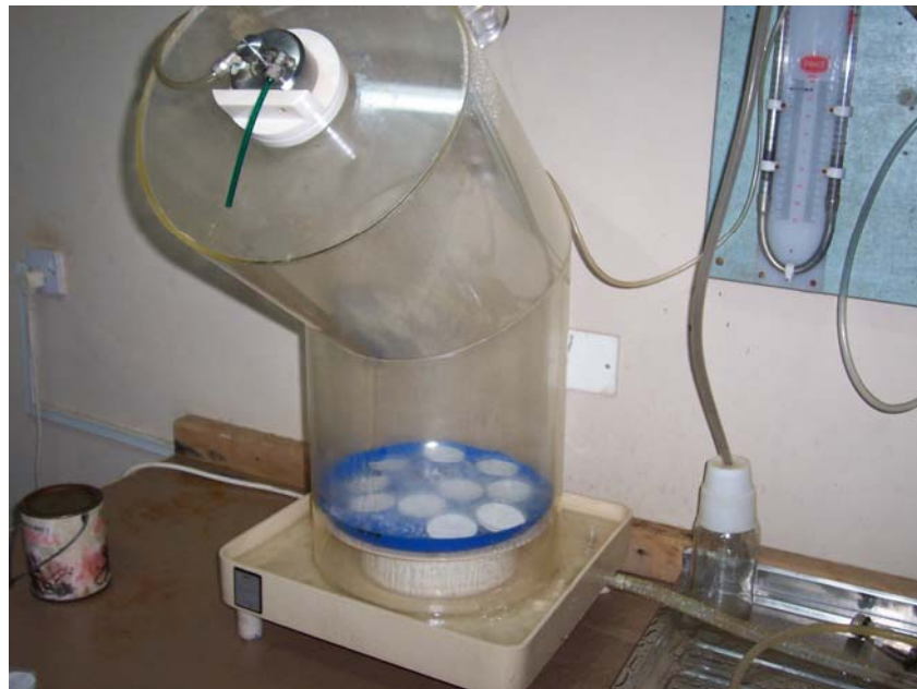
Figure 3.2 Burgerjon's spray tower used for infecting Rhipicephalus pulchellus in the laboratory
