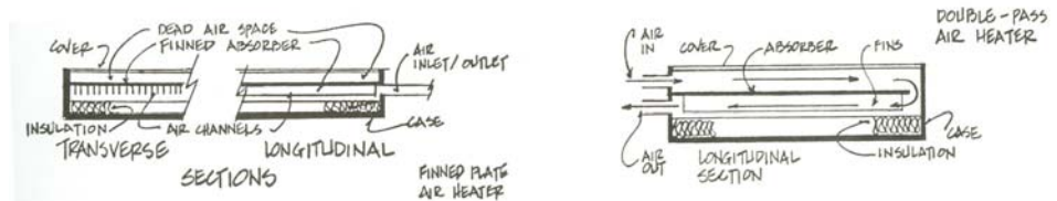
Fig 9: Air type collectors for passive air heating system.
