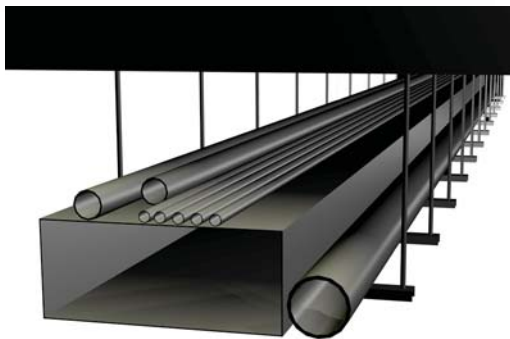
Illustration 8.2 Exposing overhead service tray through removal of first floor ceiling
