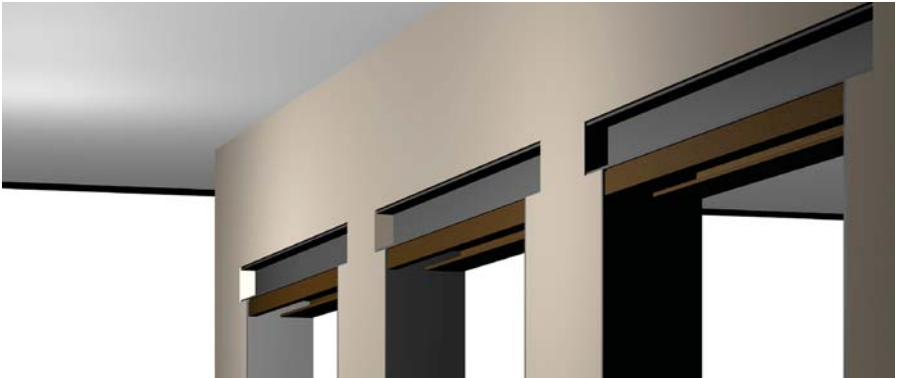
Illustration 8.1 Structural intervention after new wall penetration.
