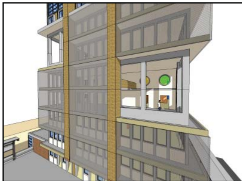
fig.10.70. Structural steel allow for vertical gardening. The proposed double volume opening connects both open-air learning areas
