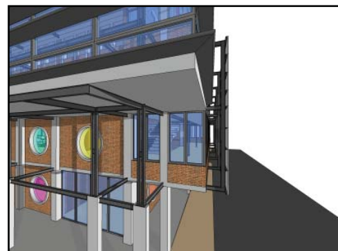
fig.10.17. I-Beam steel structure tied to building with corrugated iron sheets to form western screening device
