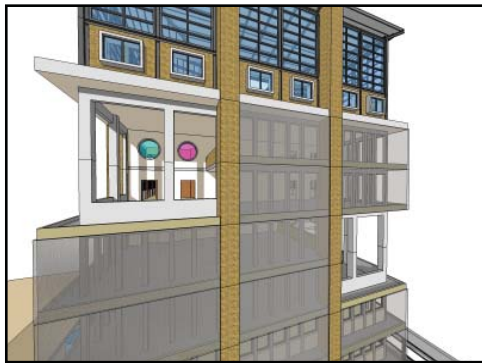
fig.10.84. Structural steel allow for vertical gardening. The proposed double volume opening connects both open-air learning areas
