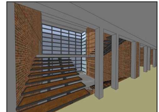
fig.10.42. Steel staircase structure with protruding glass boxes on the southern facade
