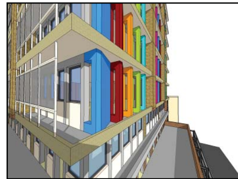
fig.10.65. Colorful angled walls to provide western screening. Northern screening provided by new glazed panels allowing for ventilation
