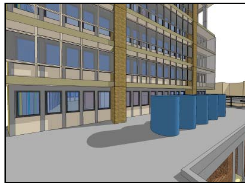
fig.10.57. Water collection tanks to provide grey water for ablution facilities below
