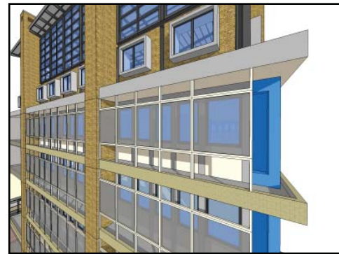
fig.10.86. Colorful angled walls to provide western screening. Northern screening provided by new glazed panels allowing for ventilation
