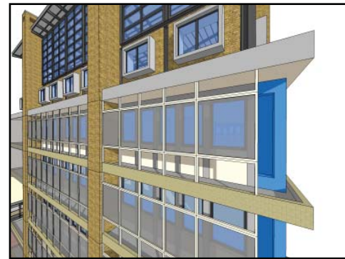
fig.10.93. Colorful angled walls to provide western screening. Northern screening provided by new glazed panels allowing for ventilation
