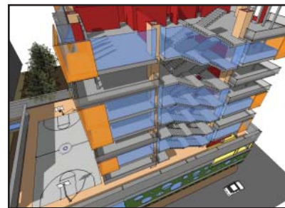
fig.9.40. New vertical circulation on northern facade
