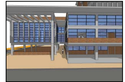
fig.9.82. Increased volume allows more natural light to reach pedestrian arcade on ground floor
