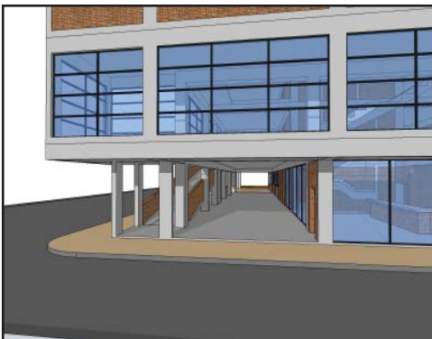
fig.9.85. Opening of structure to widen pedestrian route at Church Street interface to create safe passive surveillance area
