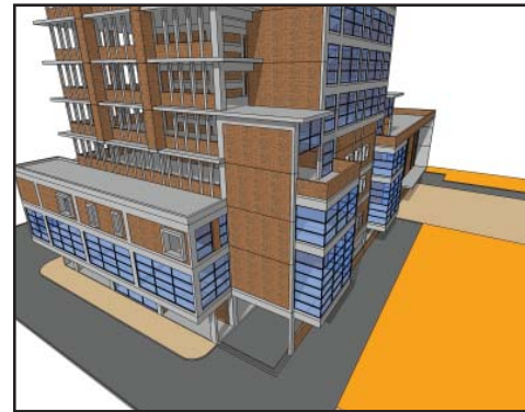
fig.9.84. New vertical circulation introduces at the lower floors on the southern facade
