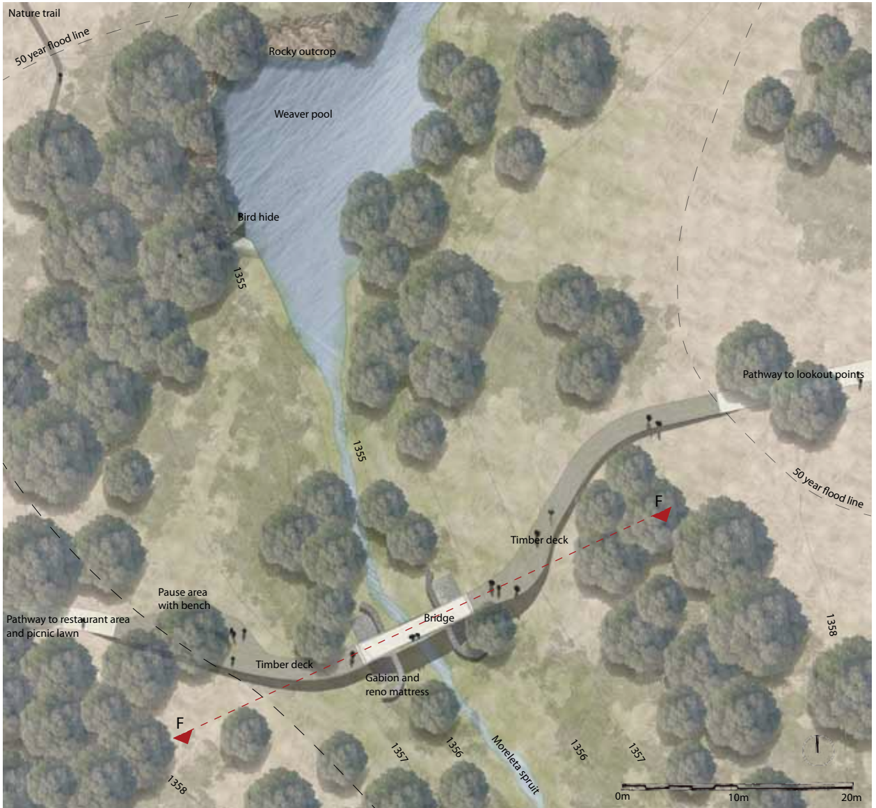
Figure 6.45 Deck and bridge sketch plan
