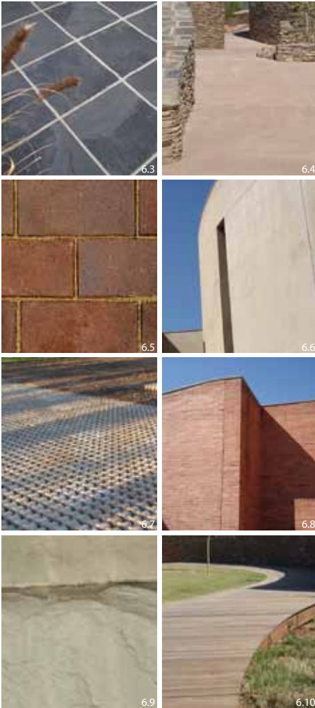
Figure 6.3 Black slate Figure 6.4 Exposed aggregate paving Figure 6.5 Nutmeg clay brick paver Figure 6.6 Off-shutter concrete Figure 6.7 Precast concrete grass block Figure 6.8 Red clay brick Figure 6.9 Sandstone tile Figure 6.10 Timber decking
