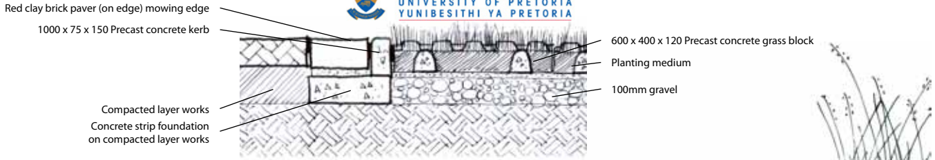
Figure 6.23 Detail A1 - Paving connection Scale 1:20
