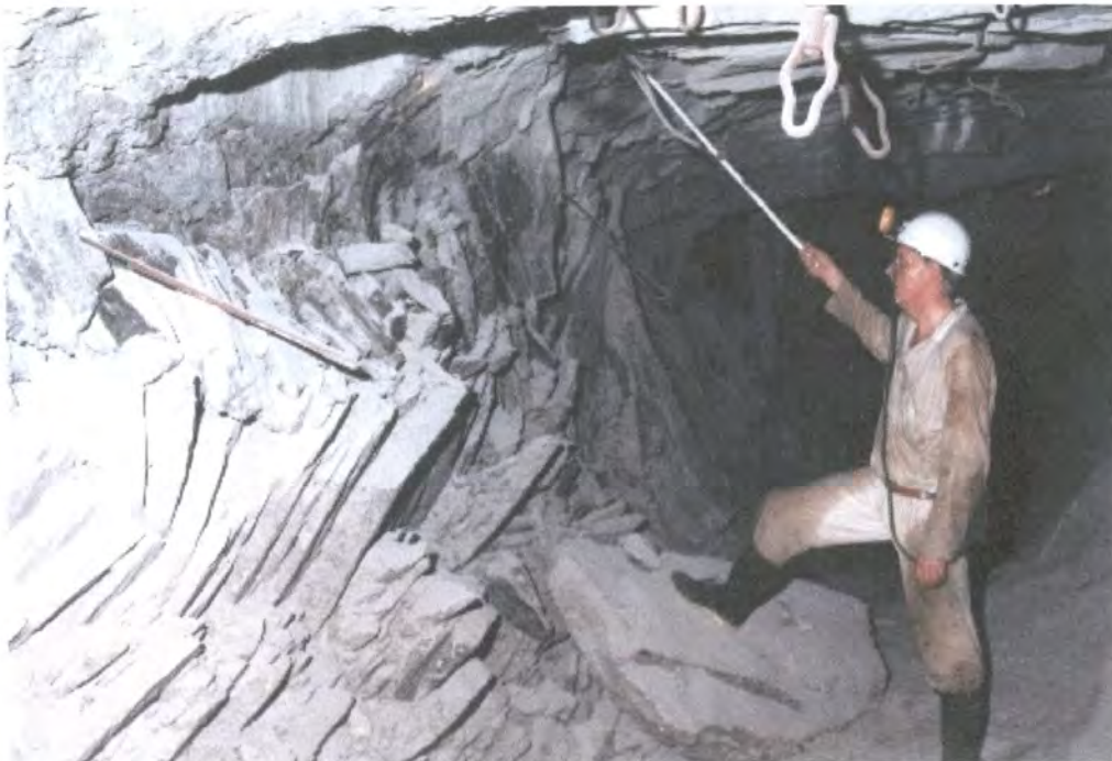
Figure 4.14 - Crush pillar directly adjacent to a gully (with no siding) is yielding in response to stope closure, resulting in slabbing being pushed, or toppling, into the gully – Merensky Reef 700 m depth
