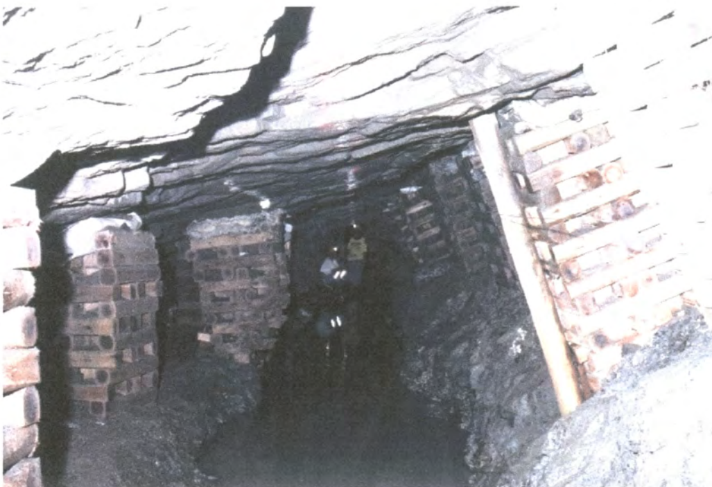
Figure 4.21 - Gully with lagging siding. Down dip siding has a flat floor due to stress fracture damage. Down dip packs are vertical
