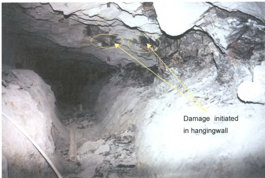
Figure 4.16 – Merensky Reef showing a short, 0.5 m siding blasted concurrently with gully advance using a single corner hole
