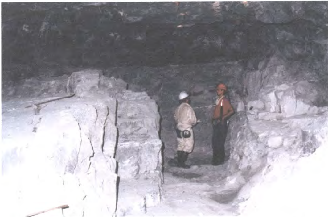
Figure 4.10 - Gully cut in a high stope width area in competent, jointed strata on the Beatrix reef at approximately 900 m depth. The gully is in the centre of a panel mining high channel widths, and is very stable, tending to break out along joint planes
