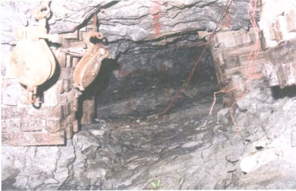
Figure 4.44 – View into a Carbon Leader wide heading showing the face charged up and ready to blast. The cut is out of sight on the up dip side. Good conditions exist over the gully
