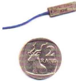
Fig A.2: The PCB piezoelectric strain gauges used on the EFBDS.
