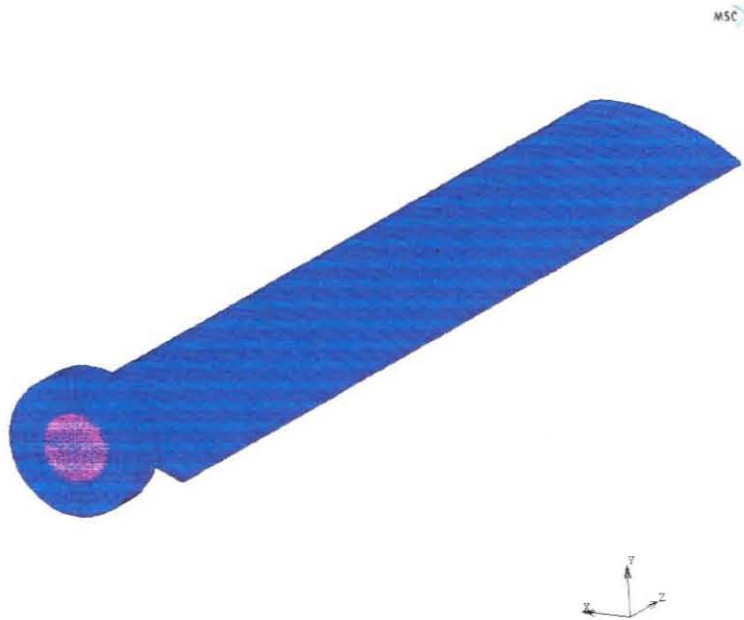
Figure 2.10: Boundary conditions (purple) for the FEM of the FD-fan blade.
