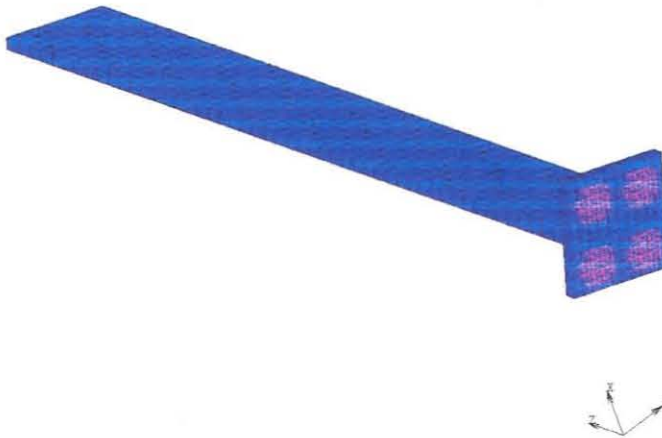
Fig 2.6: More accurate FEM for fan blade damage simulator.
