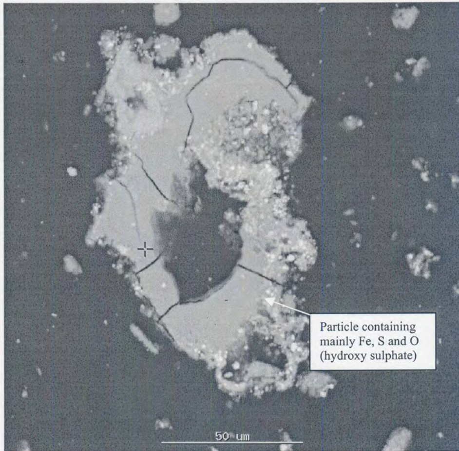
Figure 19: SEM image of an iron-bearing particle containing sulphur. Sample taken from the overflow launder of the fourth precipitation tank. (Backscattered mode)
